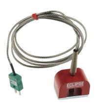
Strong 9kg pull magnet housing type K thermocouple.
