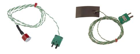
Locating a thermocouple on a surface can be achieved in various ways including the use of an adhesive patch, a washer and stud, a magnet for ferrous metals and pipe clips. Examples of surface sensing thermocouples are shown above.
