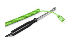
Stainless steel sheath with a moulded handle and 1.5 metres of coiled extension cable terminated in a miniature thermocouple plug. Maximum Temperature 400°C.
